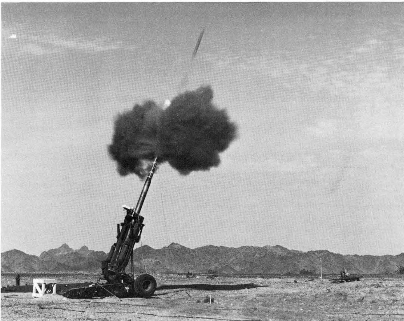
DRAMATIC PHOTO taken by David Abrahams (8186) shows firing of a W82 Joint Full Function artillery shell at Yuma Proving Grounds. Shell reached an angular acceleration of 16,000 rpm.
